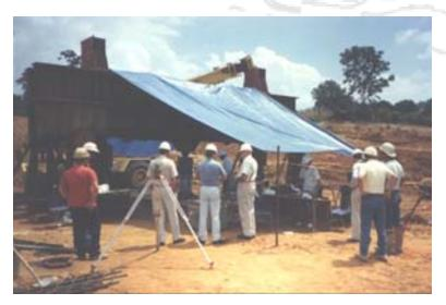
The assumption is made that the Type 3 Load Test will be carried to failure in order to justify the use of the instrumentation. The Type 3A Load Test will employ a reduced amount of internal instrumentation and has the limited aim of indication the portion of the load at failure carried in side resistance (skin friction) and in end bearing. The Type 3B Load Test will employ a sufficient amount of internal instrumentation of develop a family of curves showing the distribution of
