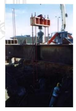
extensometers are used in order to obtain an average movement in case tilting occurs as load is applied.
